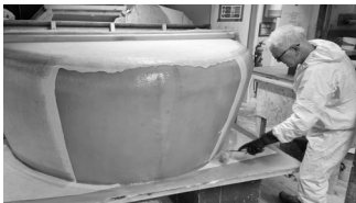
Moulding in fibreglass
