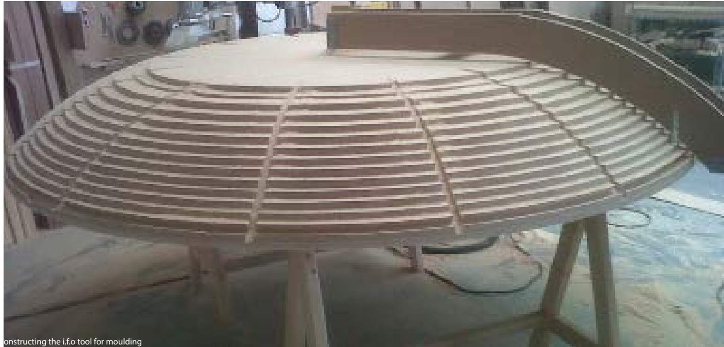
Constructing the i.f.o tool for moulding
